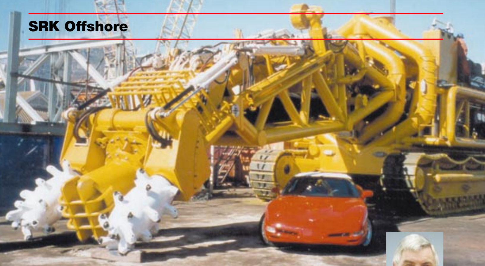
Undersea mining unit used to extract sediments from the sea floor
