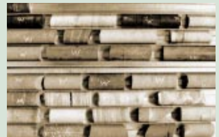
The kimberlite core samples above are shown below after only 3 wetting and drying cycles – many with extensive deterioration
