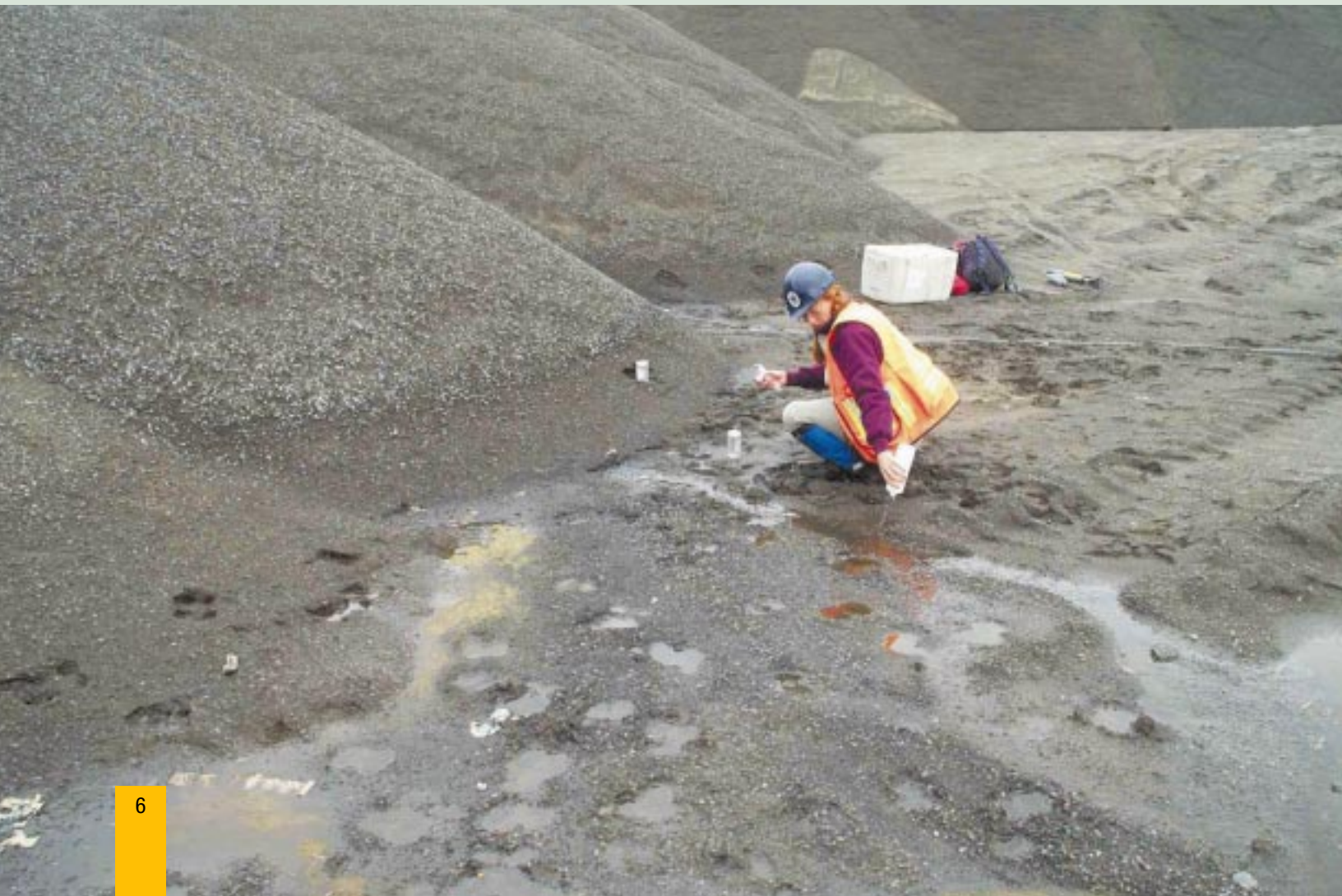
SRK's Kelly Sexsmith sampling seepage from coarse kimberlite rejects at the Ekati Diamond Mine™
